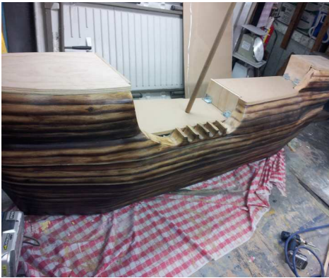
Top section begins with a 1/2 inch plywood.
